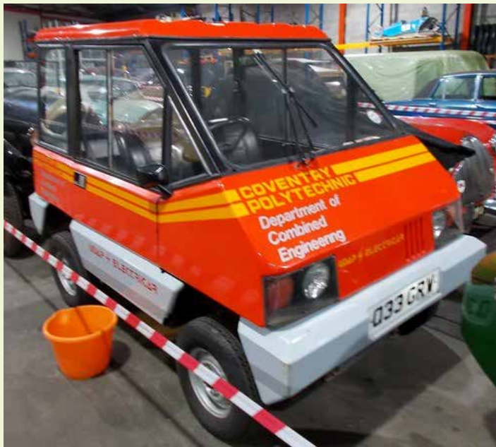
Electric Vehicle made by the Unit for the Development of Alternative Products at Coventry Polytechnic.
